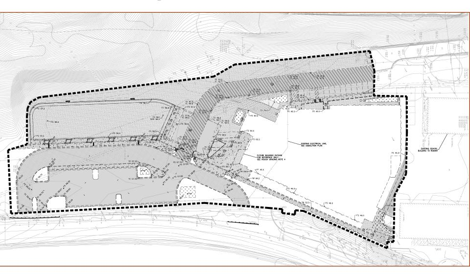
South end of site fully dedicated to construction, including utilities, staging, layout, parking. Contractor access off of Crockett Blvd.
